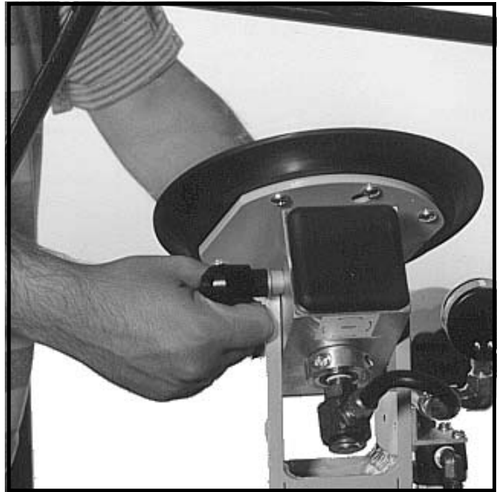
Full 360-degree edgewise rotation. One lever gives precise rotation control from light drag to lock.
